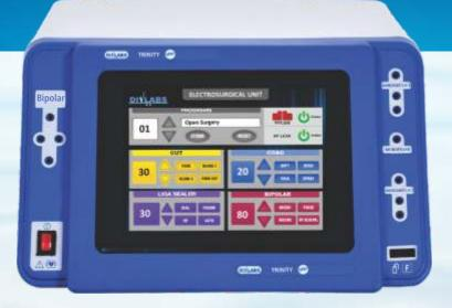
Advanced Electrosurgical system with Large Intuitive Touch Screen which provides consistent performance by using latest and reproducible technology used to command the functionality as the need of surgical application. It comes with ten programs for different specialities. 100 on site program facility possible. Three different modes of cut, coag and bipolar can be stored individually in each program. Audio Visual POP UP alarms for different conditions.
